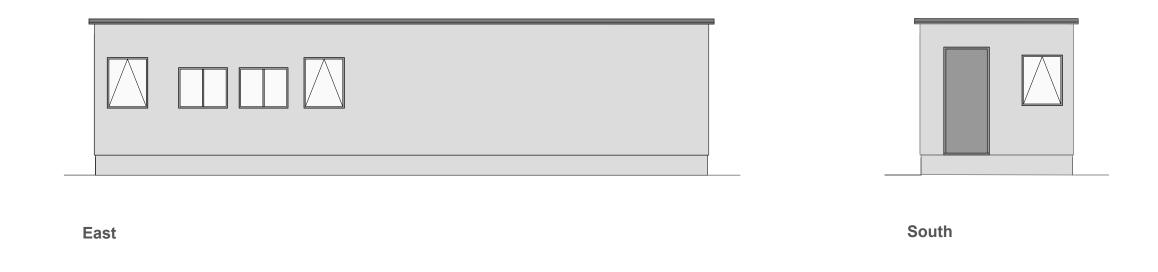
Building type - factory assembled containerised office.
